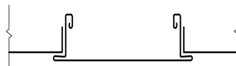
Fig. 10 – Example for a lay-on post-cap system
