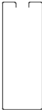
Fig. 26 – Example for a double-walled baffle made from bent or roll formed metal.
